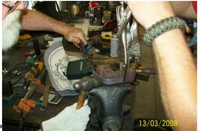
Brian Swink and Fred Connell making the Guard for a Civil War style D-Guard knife on a bending fixture that I brought that I use in my shop.
