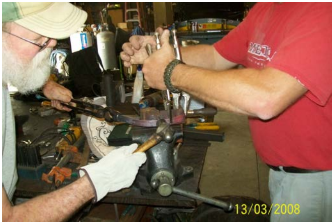
Brian Swink and Fred Connell making the Guard for a Civil War style D-Guard knife on a bending fixture that I brought that I use in my shop.
