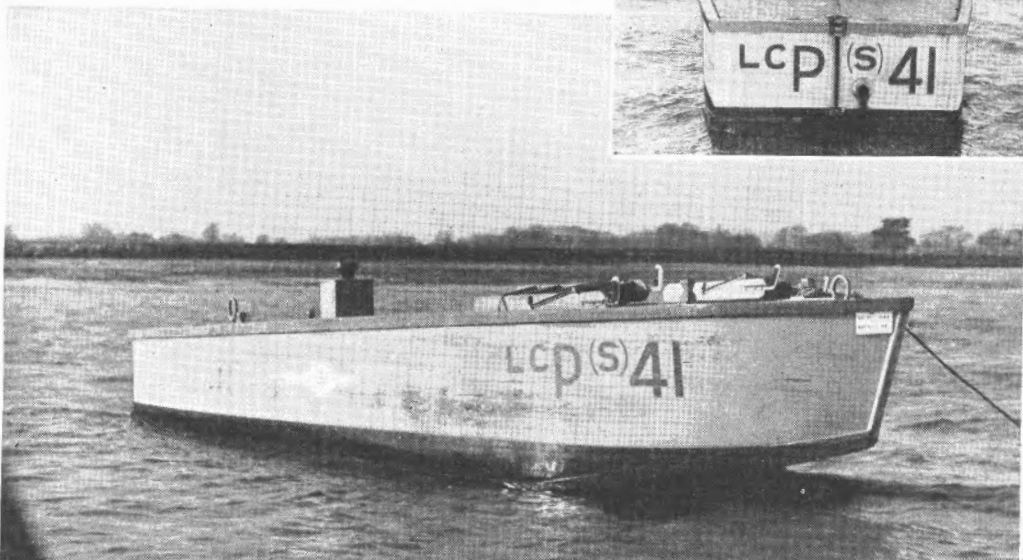
Photo shows troop benches, propeller tunnel. ▶
