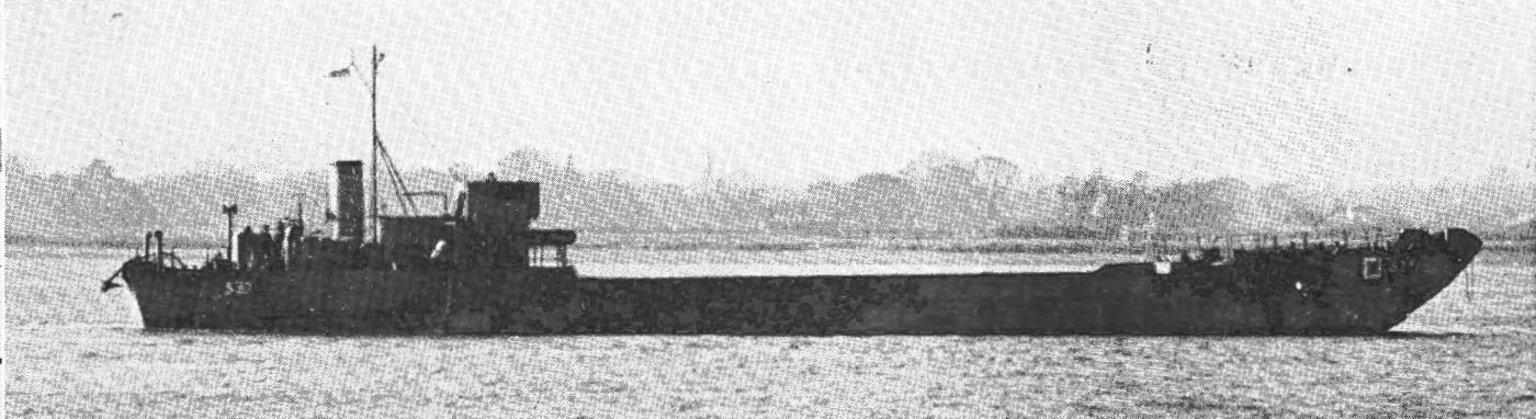
LCT(4) differs from previous models in deckhouse arrangement aft. Note steel doors in hold at the bow. ▼
