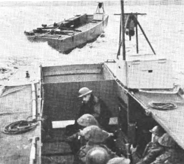
LCA Variations in the 1/4" steel doors and the bow gunners' cockpit are apparent in the photos. Note the general similarity of this design to the LCVP and LCP(R).
