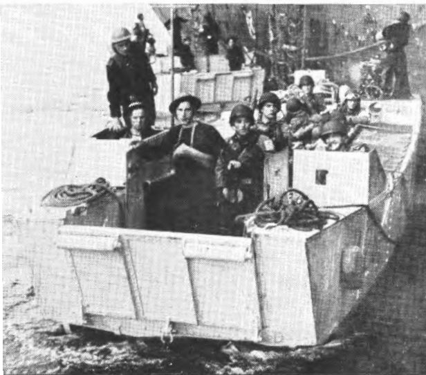
LCA Variations in the 1/4" steel doors and the bow gunners' cockpit are apparent in the photos. Note the general similarity of this design to the LCVP and LCP(R).
