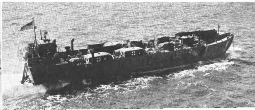
▼British units with portable ramp extensions, heightened deckhouse. Other views show recent 20 mm. additions on stern.
