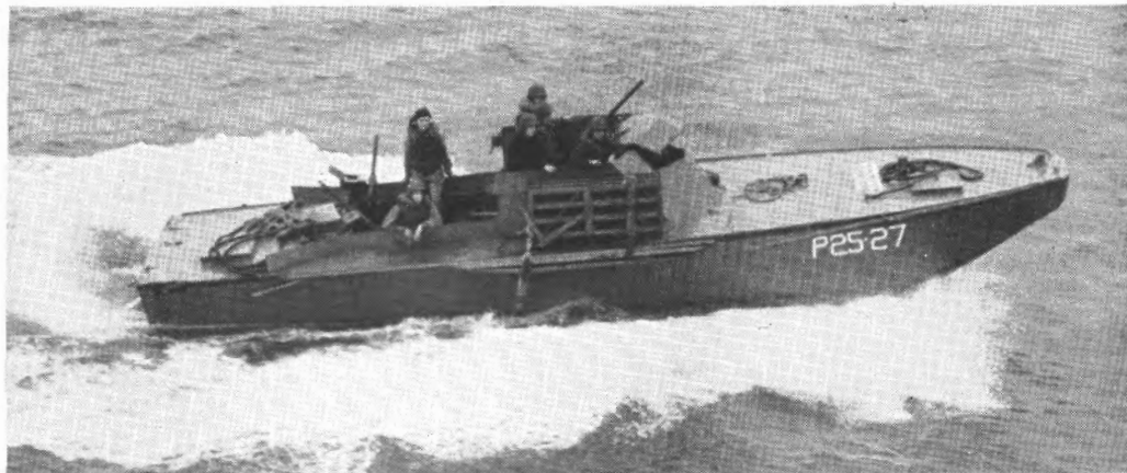
Photos Show Mark 1 With and Without Armament. Note Stern Smoke Pots.
