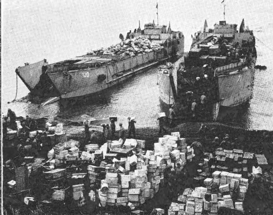
▼British units with portable ramp extensions, heightened deckhouse. Other views show recent 20 mm. additions on stern.
