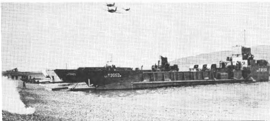
▼British units with portable ramp extensions, heightened deckhouse. Other views show recent 20 mm. additions on stern.
