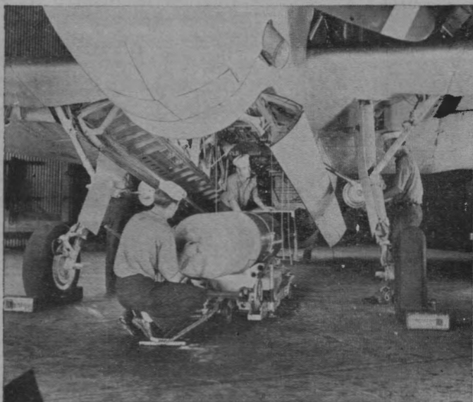
Figure 40.—Hoisting a torpedo into the bay of the TBF-1.
