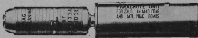
Figure 16.—A 23-lb. fragmentation bomb. The tube at the rear is the parachute case.
