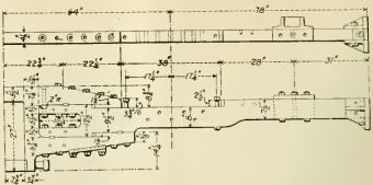
FRAME CONSTRUCTION AT CYLINDERS.
