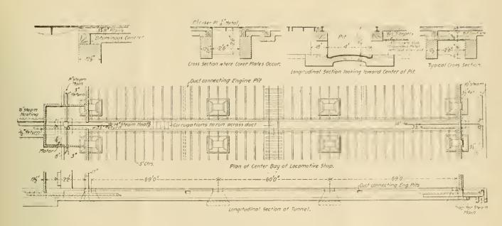
PLAN AND SECTIONS OF PIPE AND CABLE TUNNELS.
