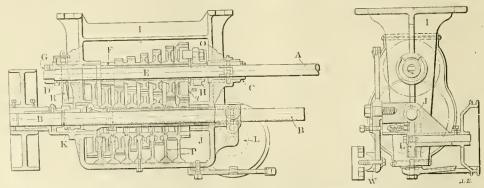
TIG. 30.—LONGITUDINAL SECTION AND CROSS SECTION THROUGH SHIPPER MECHANISM.
