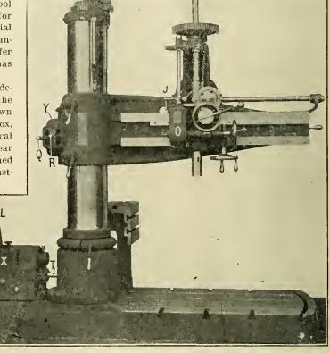
fig. 21.—the bickford radial drill. Equipped with variable-speed geared drive and feed.
