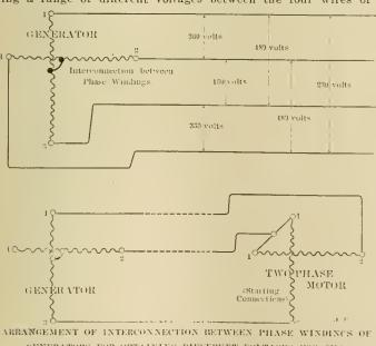
GENERATORS FOR OBTAINING DIFFERENT VOLTAGES FOR SYS-TEM OF STARTING THE MOTORS
