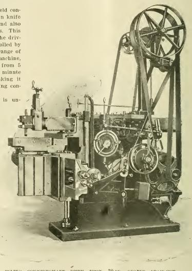
BELTED COUNTERSHAFT DRIVE UPON 30-IN, GEARED DRAW-CUT SHAPER.—MORTON MANUFACTURING COMPANY.
