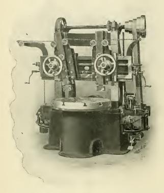
37-1N, BORING MILL.—BULLARD MACHINE TOOL CO.
