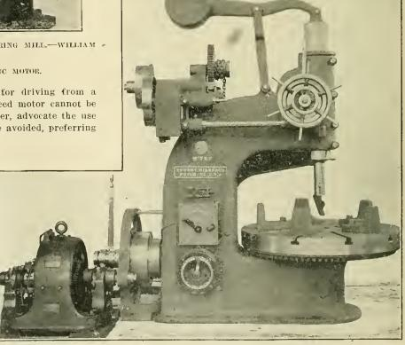
GEARED DRIVE UPON A 45-IN, CAR-WHEEL BORING MILL.—BEMENT, MILES & CO.
