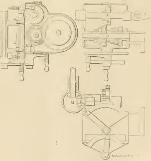
FIG. 11.—SECTIONAL VIEWS OF LOWER EIGHT-SPE D MECHANISM.
