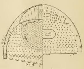
SECTION AND ELEVATION OF FIREBOX.
