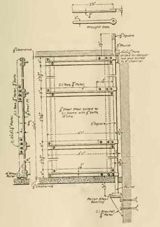
DETAILS OF BY-PASS DAMPER IN BREECHING AT ENTRANCE TO THE ECONOMIZER, SHOWING ARRANGEMENT OF ROLLER BEARING.
