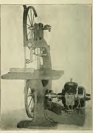
DIRECT-CONNECTED DRIVE ON 36-IN, BAND SAW, -- S. A. WOODS MACHINE COMPANY.
