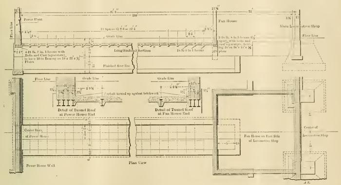
DETAILS OF THE PIPING AND WIRING TUNNEL BETWEEN THE POWER HOUSE AND LOCOMOTIVE SHOP.
