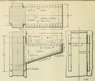
DETAILS OF STRUCTURAL STEEL BRACKET FOR SUPPORT OF MOTOR IN
