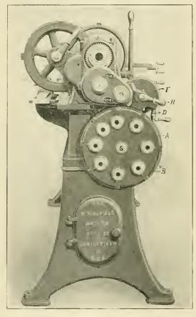
FIG. 5.—END VIEW OF IDEAL LATHE SHOWING METHOD OF SUPPORTING CHANGE GEARS BY THEIR HUES.
