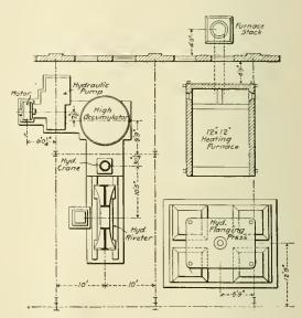
PLAN OF FLOOR UNDER RIVETING TOWER.
