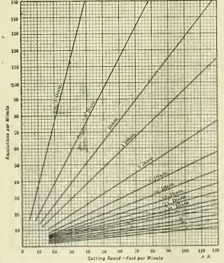
FIG. 3.—CHART INDICATING SPINDLE SPEEDS NECESSARY FOR DE-SIRED CUTTING SPEEDS WITH WORK OF VARYING DIAMETERS.
