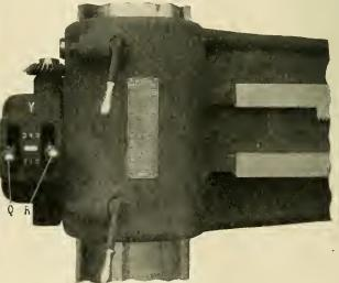
FIG. 24.—VIEW OF THE DACK GEAR BOX ON THE ARM. THIS MECHANISM IS DRIVEN THROUGH A SPLINED SHAFT AT THE REAR OF THE COLUMN.
