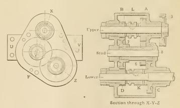
FIG. 18.—THE FOUR-SPEED CHANGE GEAR MECHANISM.
