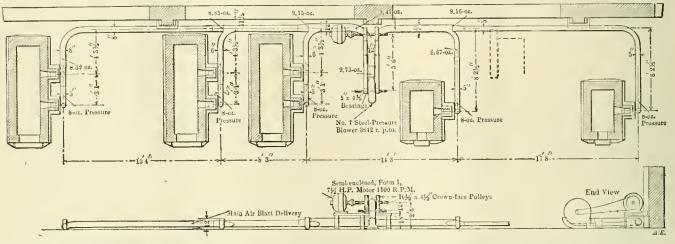
ARRANGEMENT OF THE MOTOR-DRIVEN PRESSURE BLOWER OUTFIT AND THE PIPING SUPPLYING AIR BLAST TO THE OIL FURNACES.
