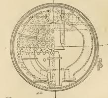
SMOKEBOX ELEVATION, SHOWING SUPERHEATER TUBES.
