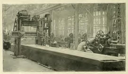
HEAVY 54-INCH X 54-INCH X 32-FOOT FRAME PLANER. —POND MACHINE TOOL CO. SPECIAL FLYWHEEL DRIVE FROM A 20-H.P. CONSTANT-SPEED CROCKER-WHEELER MOTOR. (Horizobtal Boring Machine in background at right.)
