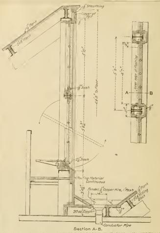
HORIZONTAL SECTION THROUGH SAW-TOOTH WINDOWS, AND VEBTICAL SECTION, A.B, SHOWING SAW-TOOTH CONSTRUCTION.
