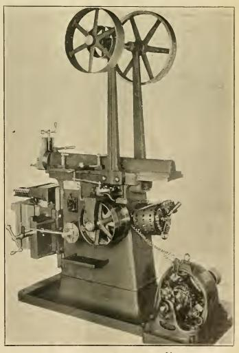
NOVEL BELTED DRIVE WITH FLY-WHEEL UPON A 24-IN, BACK SHAPER. JOHN STEPTOE SHAPER COMPANY.
