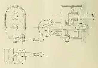
FIG. 8.—SECTIONAL VIEWS OF UPPER TWO-SPEED MECHANISM.
