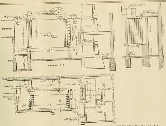
SECTIONAL DRAWINGS AND PLAN OF ECONOMIZER, SHOWING CONNECTIONS BY LOUVEE DAMPERS WITH THE EXHAUST FANS.
