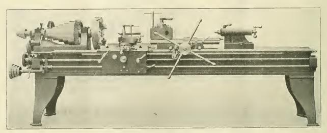
A NEW DESIGN OF ENGINE LATHE, WITH AUTOMATIC POWER-FEED TURRET ATTACHMENT.
