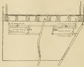
ARRANGEMENT OF PIPING USED IN THE TESTS.
