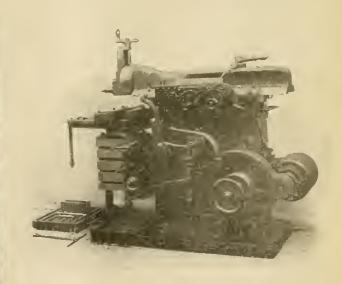
VARIABLE-SPEED GEARED DRIVE UPON THE "QUICK-STEOKE" SHAPER . BUILT BY GOULD & EBERHARDT.
