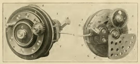
FIG. 13.—GENERAL VIEW OF THE SCHELLENBACH FEEDING ATTACHMENT.
