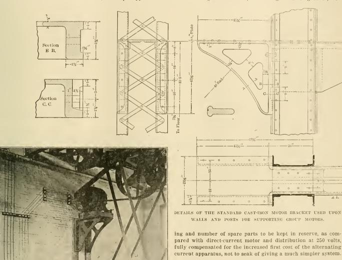
VIEW OF GROUP MOTOR AND WIRING TO STARTING SWITCH, SHOWING USE OF STANDARD MOTOR BRACKET-RATTLER GROUP IN FOUNDRY.
