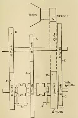
FIG. 9.—ARRANGEMENT OF GEARING FOUND NECESSARY ON A 25-IN. PUTNAM LATHE.
