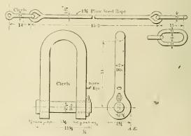
DETAILS OF THE CLEVIS FOR A STEEL ROPE SLINO.
