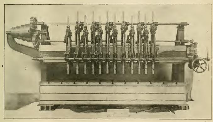
NEW 12-SPINDLE MUD RING DRILLING MACHINE.
