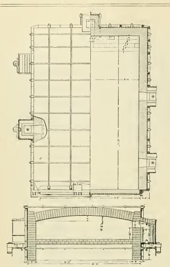
PLAN AND SECTIONAL ELEVATION OF THE ANNEALING AND FLANGINO FURNACE.
