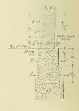
STANDARD SECTION FOR SIDE AND END FOUNDATIONS,
