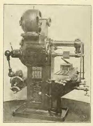
FIG. 1.—VARIABLE-SPEED DRIVE FOR A UNIVERSAL MILLING MA-CHINE, ALL PARTS ENCLOSED—CINCINNATI MILLING MA-CHINE COMPANY—CBOCKER-WHEELER MOTOR.
