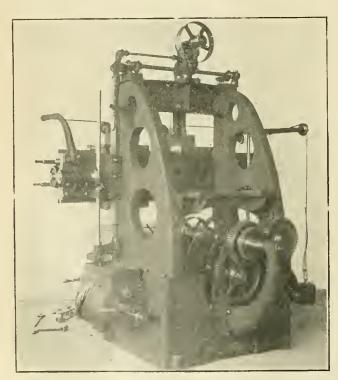
REAR VIEW OF THE 41-IN. BAUSH DORING MILL, SHOWING ARRANGE-MENT OF BRACKET BETWEEN FRAMES FOR SUPPORTING MOTOR.
