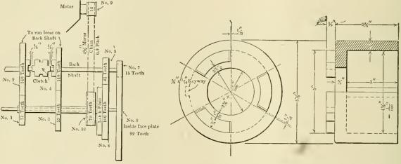
FIG. 11.—ARRANGEMENT OF GEARING UPON A 42-1N. NILES TRIPLE-GEARED LATHE.
