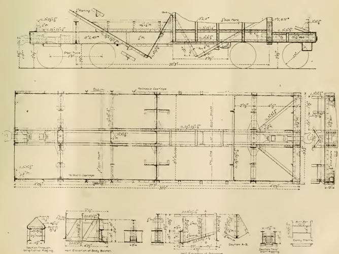
DETAILS OF THE ABOVE STRUCTURAL HOPPER CAR, CARNEGIE DESIGN, RUILT BY THE SCHOEN PRESSED STEEL CAR CO.
