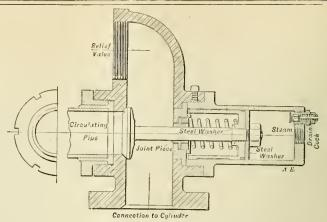
FIG. 3.—DETAILS OF RELIEF VALVE.
