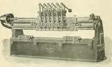
NEW 6-SPINDLE MUD-RING AND FLUE-SHEET DRILL. WITH AUXILIARY CROSS RAIL. FOOTE, BURT & CO.
