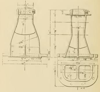
DETAILS OF THE FOUR-CHAMBER EXHAUST PIPE.
