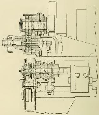
FIG. 6 — SECTIONAL VIEW OF IDEAL LATHE GEAR-ROX, SHOWING CLUTCH ARRANGEMENT.
