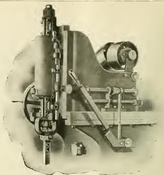
SHOWING DEVICE FOR CHANGING DEPTH OF MORTISE, ALSO, LAYOUT STOPS
