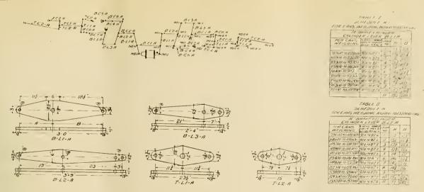
foundation brake for passenger cars, with high-speed brakes. schedules a and a-1, cars weighing 80,000 to 137,000 lbs. 6-wheel trucks.
