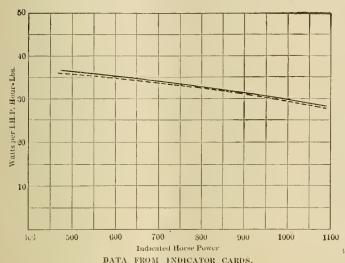
(DOTTED CURVE REPRESENTS THE PISTON-VALUE ENGINE, AND SOLID CURVE THE SLIDE-VALUE ENGINE.)
