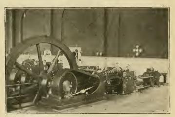
THE TWO-STAGE, CROSS-COMPOUND AIR COMPRESSOR.—INGERSOLL-SERGEANT DRILL COMPANY.
