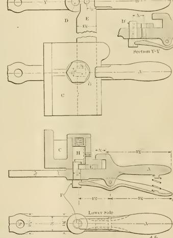
FIO. 8.—DETAILS OF CLUTCH HANDLE INTERLOCKING MECHANISM.
