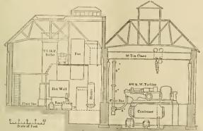
SECTIONAL ELEVATION OF BOILER AND ENGINE
