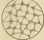
Figure One—Ferrite crystals containing no carbon.
