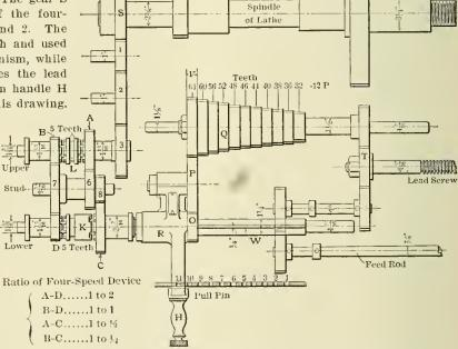
FIG. 20.—DIAGRAM ILLUSTRATING PRINCIPLE OF THE DRIVE THROUGH BOTH MECHANISMS.
