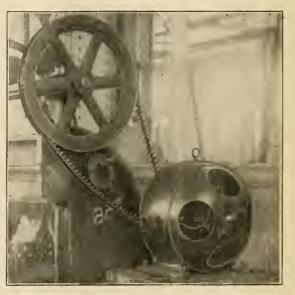
VIEW OF A CHAIN DRIVE UPON A MACHINE TOOL.
