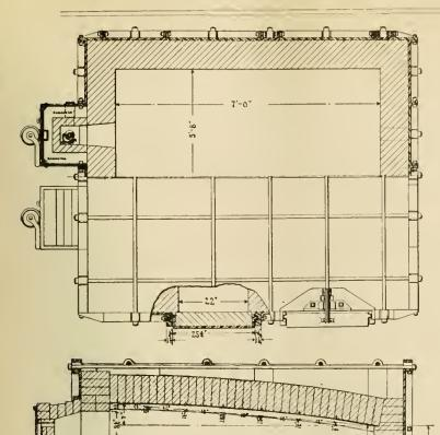
PLAN AND SECTIONAL ELEVATION OF THE LARGE FORGING FURNACE.
