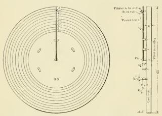
PLATE FOR LAYING OUT DUNBAR PACKING RINGS.
