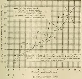
FIG. 1.—DIAGRAM SHOWING RELATION BETWEEN THE SPEED AND POWER OF A MOTOR USING THE M. F. 21 (FIELD WEAKENING) CONTROLLER.
