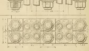
DETAILS OF THE ATTACHMENT OF THE SUPERHEATER TUBES TO THE HEADER.
