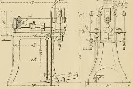
FERGUSSON'S PNEUMATIC FLUE WELDING MACHINE.
