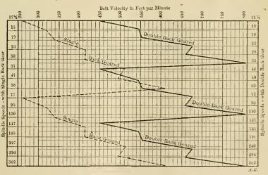
FIG. 38.—DIAGRAM SHOWING INCREASED BELT VELOCITY PROVIDED IN THE DOUBLE BACK-GEARED MACHINE.
