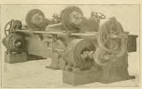
INTERESTING ARRANGEMENT OF ELECTRICAL DRIVING FOR A DOUBLE-HEAD TRAVERSE SHAPER. CINCINNATI SHAPER COMPANY.
