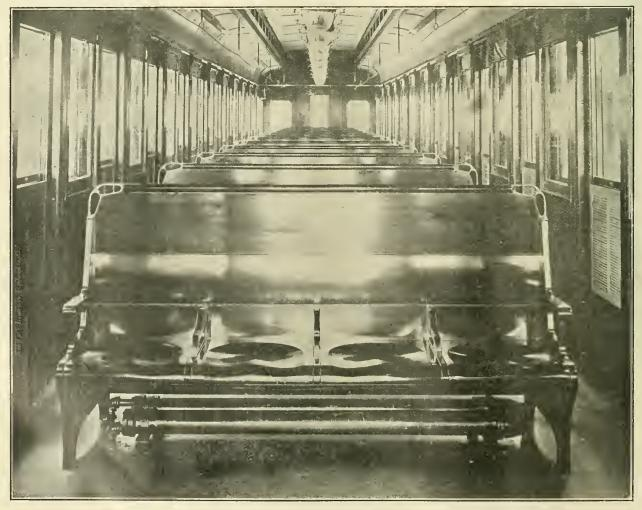
INTERIOR VIEW OF CAR, SHOWING MOULDED-FORM SEATS AND AISLE ARRANGEMENT.
