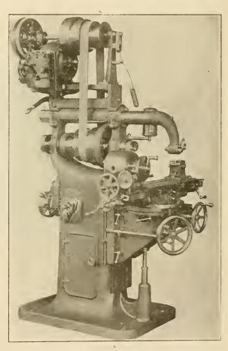
FIG. 4.—CONSTANT-SFEED DRIVE HENDY-NORTON UNIVERSAL MILLING MACHINE WITH BOTH CHANGE GEARS AND CONE PULLEYS NORTHERN ELECTRIC MOTOR.
