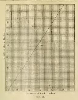
RELATION OF DIAMETER TO HEIGHT OF STACK FOR THE PURDUE EXPERIMENTAL LOCOMOTIVE FOR BEST RESULTS WHEN EXHAUST NOZZLE IS ON CENTER LINE OF BOILER.
