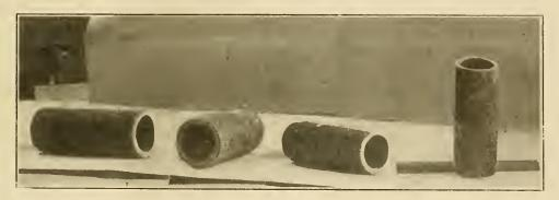
SAMPLES OF SCALED BOILER TUBES, TAKEN FROM LOCOMOTIVES OF THE PITTSBURGH & LAKE ERIE BAILROAD, AFTER 12 MONTHS OF SERVICE WITH THE UNTREATED WATER.
