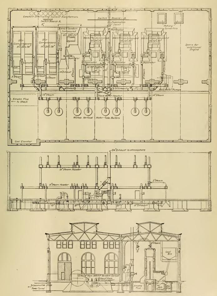
FLOOR PLAN AND CROSS SECTION OF BUILDING, AND SPECIAL SECTIONAL ELEVATION TO SHOW ARRANGEMENT OF STEAM PIPING.
