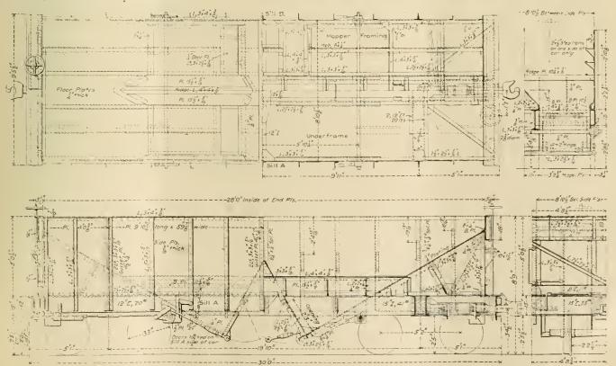
PLAN, AND SIDE AND SECTIONAL ELEVATIONS OF THE STBUCTUBAL STEEL CAR BUILT BY THE KEYSTONE BRIDGE WAR.
