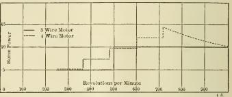
FIG. 1.—HORSE-POWER DIAGRAM FOR MOTORS ON THE 3 AND 4-WIRE
