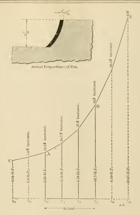
DIAGRAM OF POWER REQUIRED WITH VARYING CUTS.
