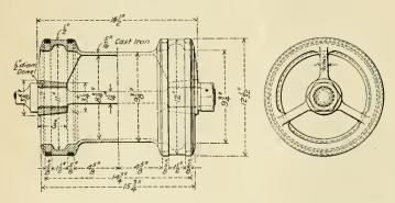
PISTON VALVE, USED FOR BOTH HIGH AND LOW PRESSURE CYLINDERS.
