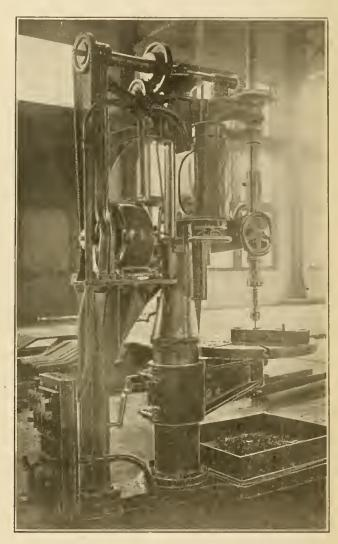
REMODELING, FOR AN FIG. 22—APPEARANCE OF THE DRILL AFTER BEING EQUIPPED WITH THE CROCKER-WHEELER MULTIPLE-VOLTAGE DRIVE.
