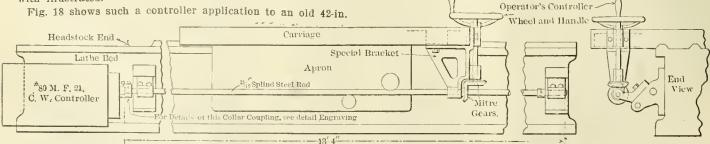
FIG. 18—COMPACT ARRANGEMENT OF MOTOR CONTROLLER (CHOCKER-WHEELER MULTIPLE-VOLTAGE SYSTEM) UPON THE 42-INCH NILES LATHE.
