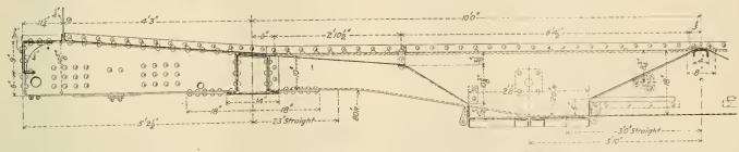
CLASS GM CAR-CENTER SILL, END SILL, BOLSTER AND DRAFT GEAR CONSTRUCTION.
