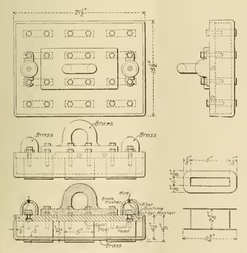
ELECTRO-MAGNET FOR HANDLING BOILER PLATE-CHICAGO & NORTHWEST-ERN RAILWAY.
