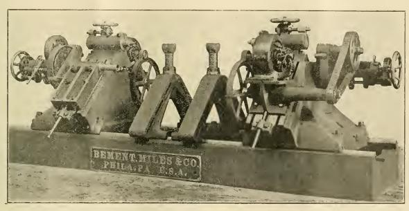
A NEW DESIGN OF ELECTRIC DRIVING FOR A QUARTERING MACHINE. DRIVEN BY A  $3\frac{1}{2}$ -11.P. CONSTANT-SPEED CROCKER-WHEELER MOTOR UPON EACH HEAD.
