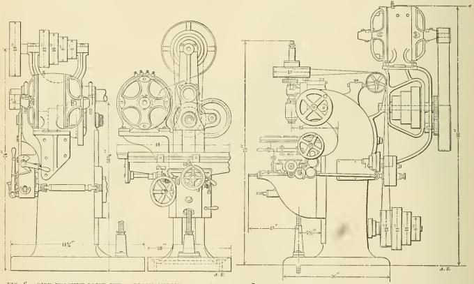
FIG. 6.—SIDE BRACKET DRIVE FOR A PLAIN MILLING MACHINE.
