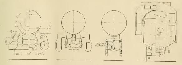
THE TRACTION INCREASER CYLINDERS ARE LOCATED IN FRONT OF FIRST AND IN REAR OF THIRD DRIVING AXLES.
