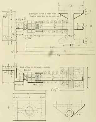
LATERAL SPRING CENTERING DEVICE FOR LOCOMOTIVE TRUCKS.
