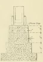
SECTION THROUGH CENTER PIER FOUNDATIONS.
