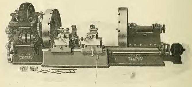
HEAVY NILES DRIVING-WHEEL LATTHE, ELECTRICALLY DRIVEN THROUGH A TWO-SPEED MAGNETIC CLUTCH.
