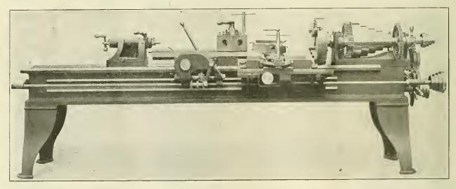
REAR VIEW OF THE LATHE, SHOWING TURRET MECHANISM AND TAPER-TURNING ATTACHMENT. GREAVES, KLUSMAN & CO.
