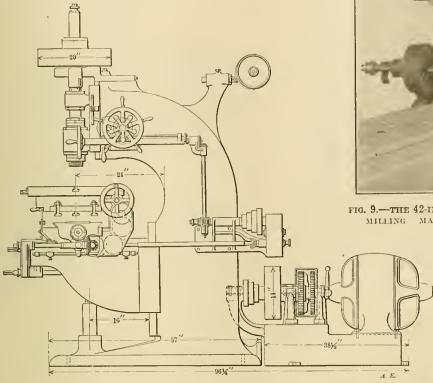
FIG. 8.—FLOOR MOTOR BRIVE AS APPLIED TO A BECKER-BRAINARD VERTICAL MILLING MACHINE.
