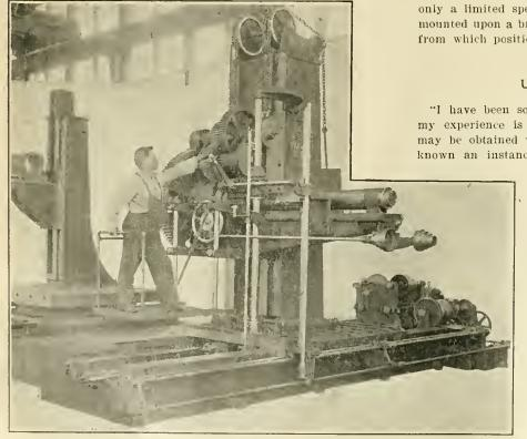
GEARED DRIVE UPON A TARGE HORIZONTAL DRILLING AND BORING MACHINE. -BEAMAN & SMITH.
