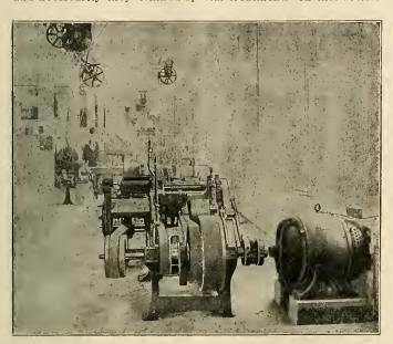
FIG. 1.—DIRECT-COUPLED DRIVE FOR A 9-INCH STICKER. DRIVEN BY
