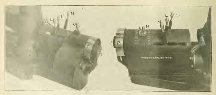
FIG. 40.—BEAR VITW OF THE SPEED BOX, SHOWING CASING FOR INTERMEDIATE GEARS,
