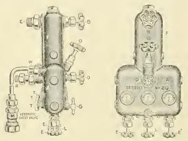
one inch thick are used for the sight feed feature all danger from broken glasses is entirely removed. As it has but very few joints the liability to leakage is slight, and as the oil is delivered to the sight feed chamber from a point within the reservoir there can be no chilling of the oil in cold weather. This lubricator is known as the "Detroit No. 20." The manufacturers will be glad to send descriptive matter to all interested.
