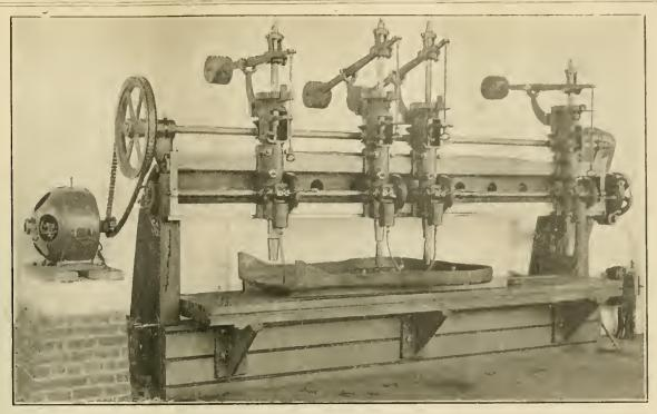
Four-spindle mud ring drill.—Niles tool works company. Driven by a  $7\frac{1}{2}$ -11.P. Multiple-voltage crocker-wheeler motor.
