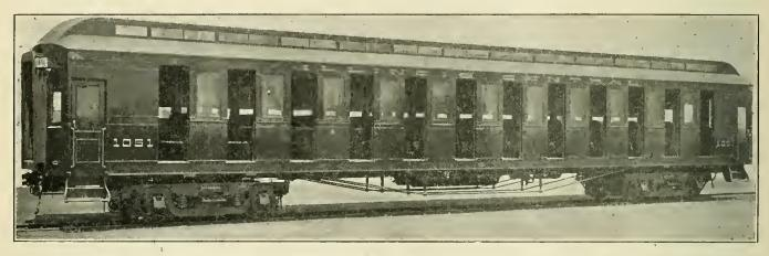
VIEW OF CAR WITH SIDE DOORS OPEN, INDICATING LARGE EXIT CAPACITY.
