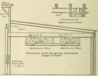
DRIVING ARRANGEMENT FOR THE GROUP LINE SHAFTS.
