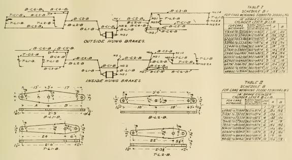
FOUNDATION BRAKE FOR PASSENGER CARS, WITH HIGH-SPEED BRAKES. SCHEDULES B AND B-1. CARS WEIGHING 50,000 to 90,000 lbs. 4-Wheel trucks.
