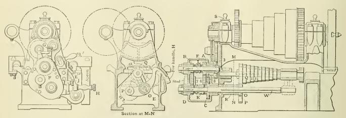
FIG. 19.—EXTERNAL END VIEW OF LATHE, AND CROSS AND LONGITUDINAL SECTIONS OF THE ELEVEN-SPEED MECHANISM WITHIN THE BED.
