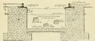
CROSS-SECTION SHOWING DETAILS OF ERECTING PIT CONSTRUCTION.
