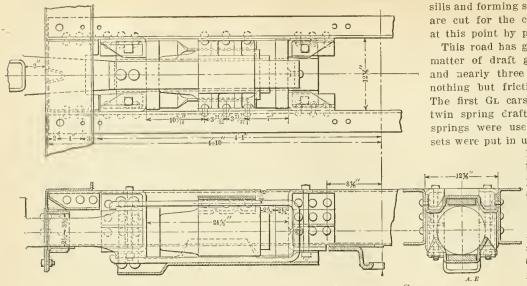
DETAILS OF DRAFT GEAR ATTACHMENT—WESTINGHOUSE—CLASS GL. CARS.
