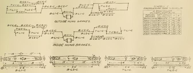
foundation brake for passenger cars, with high-speed brakes. Schedule c. . Cars weighing less than  $50,\!000$  lbs. 4-wheel trucks.
