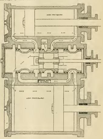
DIAGRAM OF VALVE AND CYLINDERS.
