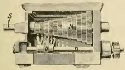
FIG. 2. REAR VIEW OF GEAR-BOX, SHOWING GEARING.
