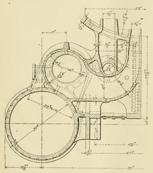
CROSS SECTION OF LOW-PRESSURE CYLINDER AND VALVE.
