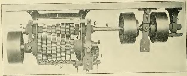
FIG. 28.—FRONT VIEW WITH COVERS REMOVED, SHOWING SHIPPER LEVER AND CONNECTING BOD TO SLOW-SPEED CLUTCH.
