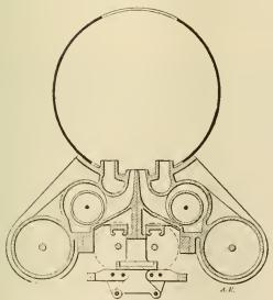
SECTION THROUGH LOW-PRESSURE CYLINDERS.
