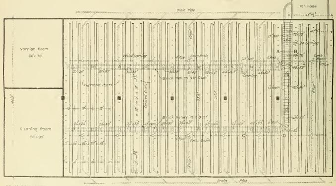
PLAN OF PASSENGER CAR PAINT SHOP, SHOWING ARBANOEMENT OF TRACKS, RETURN AIR DUCTS, DRAINS, PLATFORM POSTS, ETC.
