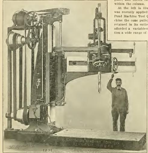
COMBINATION CHAIN AND BELTID DRIVE UPON A 6-FT RADIAL DRILL.—POND MACHINE TOOL COMPANY.
