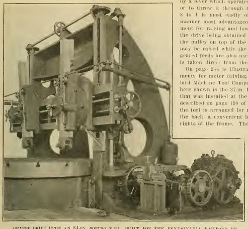
GEARED DRIVE UPON AN 84-IN. BORING MILL, BUILT FOR THE PENNSLVANIA RAILROAD BY THE BETTS MACHINE COMPANY.
