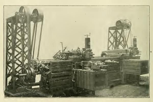
36-INCH DOUBLE-HEAD MOTOR-DRIVEN TRAVERSE SHAPER.—CINCINNATI SHAPER CO.
