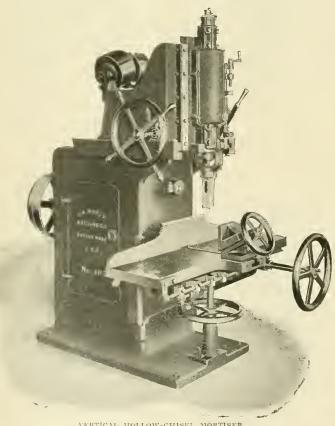
VERTICAL HOLLOW-CHISEL MORTISER.
