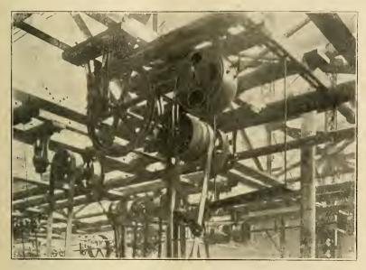
TYPICAL ARRANGEMENT OF CEILING MOTOR FOR GROUP DRIVING.
