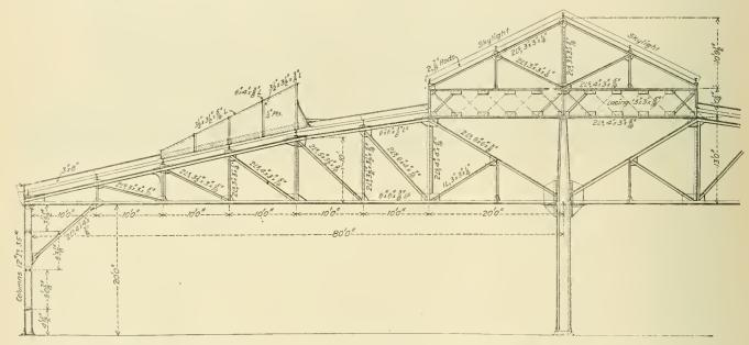
CROSS-SECTION, SHOWING STEEL CONSTRUCTION AS APPLIED TO BOTH FREIGHT AND PASSENGER DEPARTMENT BUILDINGS OF THE NEW CAR REPAIR SHOPS.
