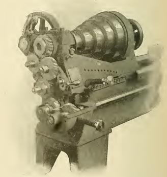
FIG. 52—VIEW OF THE HEADSTOCK END OF THE LODGE & SHIPLEY LATTIE, SHOWING ARRANGEMENT OF THE VARIABLE-SPEED FEEDING MECHANISMS.
