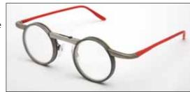
and the clear rigid surface holds a small amount of clear optical fluid. As a slider on the bridge is moved, the fluid is pushed forward to alter the shape of the membrane, which alters the flexible lens and changes its focus, mimicking the performance of the natural lens. TruFocals allow the user to adjust the focus of his lens at any distance and under any lighting condition.
